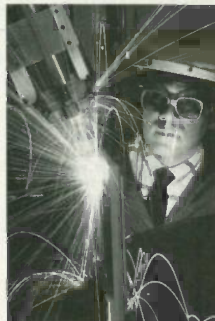
GE R&D CENTER ENGINEER ANGEL L. ORTIZ, JR puts the face-pumped laser to work drilling holes in a \frac{1}{2} -inch thick plate of superalloy; in other tests it's managed to drill through more than two inches of superalloy. The solid-state laser's average power output of 1,000 watts from a single laser head opens the door to development of industrial laser systems that can cut and drill space-age metals and alloys with unprecedented speed and precision.
